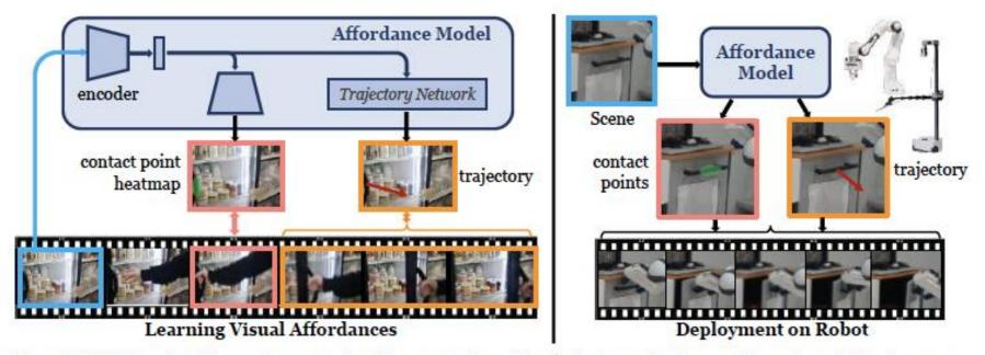
Figure 2. VRB Overview. First, we learn an actionable representation of visual affordances from human videos: the model predicts contact points and trajectory waypoints with supervision from future frames. For robot deployment, we query the affordance model and convert its outputs to 3D actions to execute.
