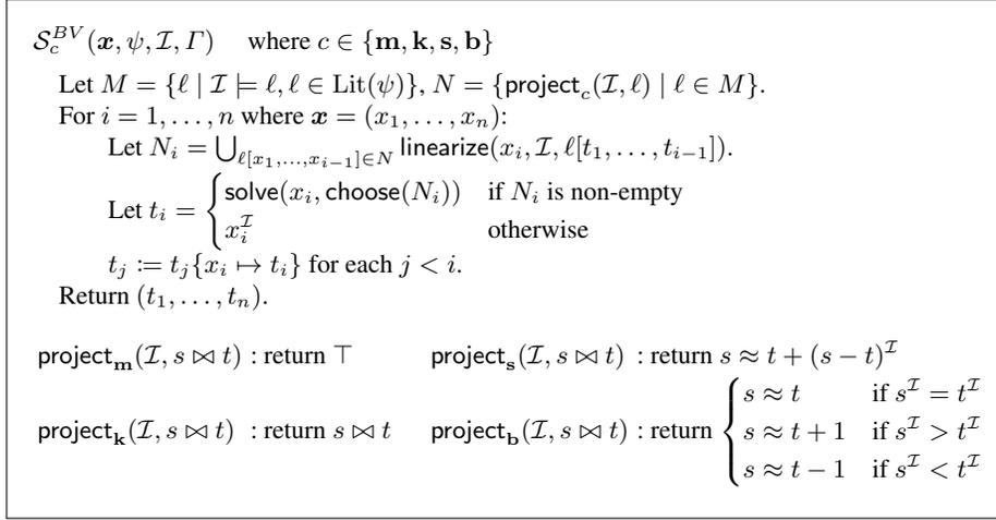
**Fig. 3.** Selection functions  $\mathcal{S}_c^{BV}$  for quantifier-free bit-vector formulas. The procedure is parameterized by a configuration  $c$ , one of either  $\mathbf{m}$  (model value),  $\mathbf{k}$  (keep),  $\mathbf{s}$  (slack), or  $\mathbf{b}$  (boundary).
