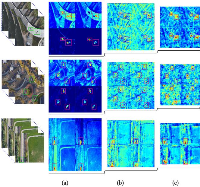
**Figure 5: Visualization of different layers in MOR-UAVNet. (a) convolutional layer before the backbone feature extraction, (b) pyramid level 3, (c) pyramid level 4. The relevant motion saliencies of moving objects are highlighted using red boxes.**
