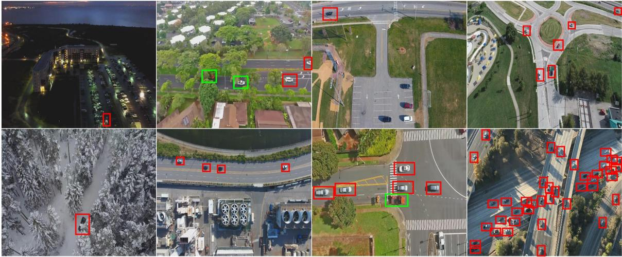
**Figure 2: Sample video frames taken from MOR-UAV. The videos are collected from different scenarios including night time, occlusion, camera motion, weather conditions, camera views, etc. The red and green boxes denote two object classes car and heavy-vehicle respectively.**
