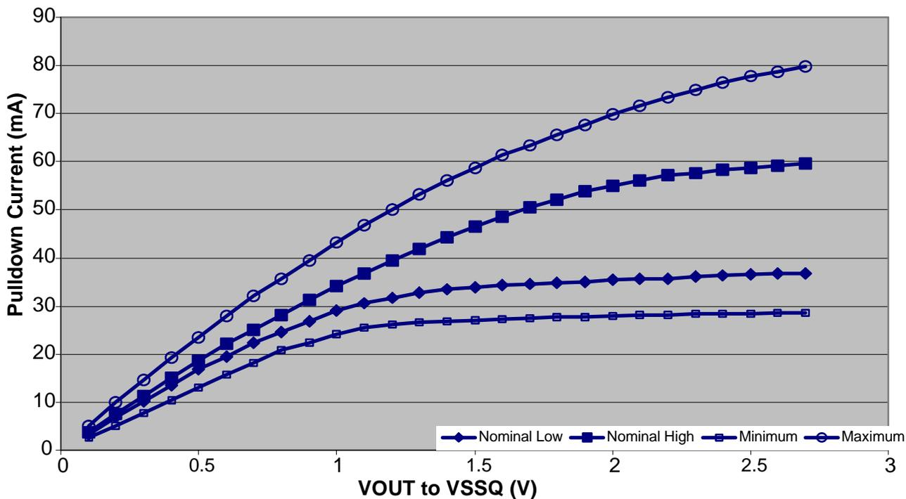
Figure 40b: Pulldown Characteristics for Weak Output Driver
