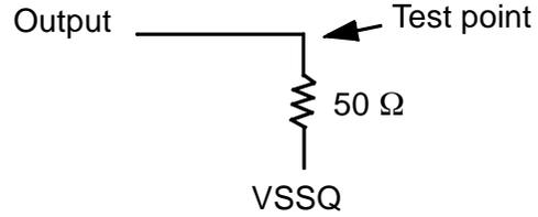
Figure 37: Pullup slew rate test load
