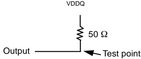
Figure 38: Pulldown slew rate test load
