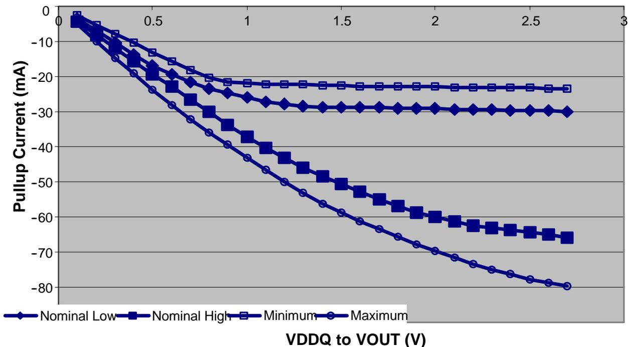
Figure 40a: Pullup Characteristics for Weak Output Driver
