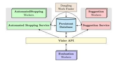
Figure 1: Architecture of Vizier service: Main components are (1) Dangling work finder (restarts work lost to preemptions) (2) Persistent Database holding the current state of all Studies (3) Suggestion Service (creates new Trials), (4) Early Stopping Service (helps terminate a Trial early) (5) Vizier API (JSON, validation, multiplexing) (6) Evaluation workers (provided and owned by the user).
