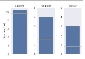
*Figure 6.* Effect of quantization polarity on the runtime of the first fire layer in SqueezeNet. The horizontal yellow line indicates the runtime of the layer if it were run with perfect efficiency.
