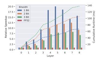
*Figure 4.* Layerwise speedup of SqueezeNet quantized with varying bitwidth versus the floating point baseline model.
