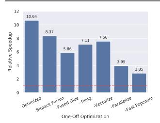
*Figure 5.* Ablation study of the effect of Riptide optimizations versus the baseline floating point model.
