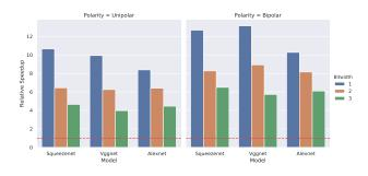
*Figure 3.* Visualization of end to end speedups of all explored models and bitwidths compared to floating point baselines.
