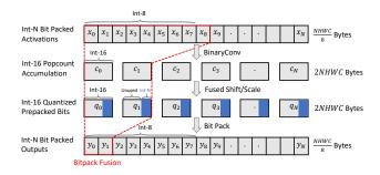
Figure 2. Scheduling of N-bit binary layer demonstrating intermediate memory used. By fusing computation within tiles, such as the region highlighted red, memory use can be reduced.
