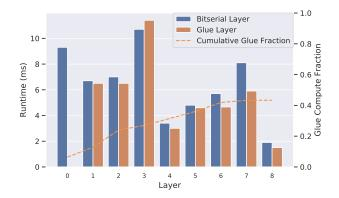
*Figure 7.* Layerwise runtime breakdown of SqueezeNet quantized with 1-bit weights and activations.
