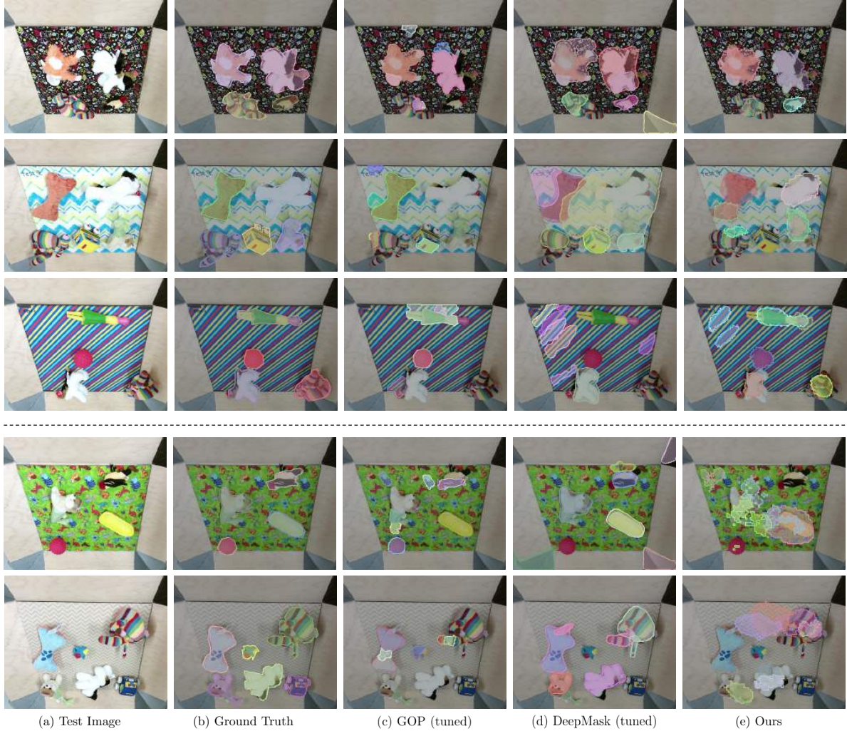
Figure 5. Visualization of the object segmentation masks predicted by a bottom up segmentation method GOP with Domain Knowledge (c; GOP tuned), a top down segmentation method trained with strong supervision using more 700K human annotated ground truth object masks (d; DeepMask) and our method (e). The top three rows show representative examples of cases when our methods predicts good masks and the bottom two rows illustrate the failure mode of our method. In general GOP has low recall. The performance of our method and DeepMask is general. Our dominant failure mode is prediction of small disconnected masks (row 4).
