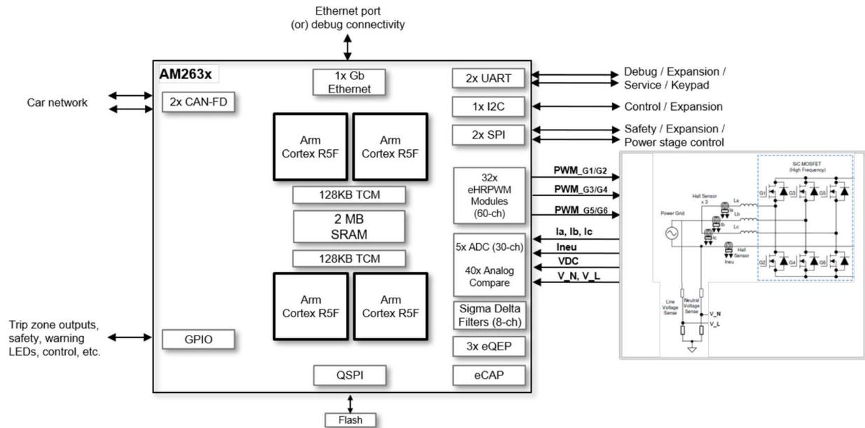
More complex AM263x power control use cases will involve partitioning of processing across R5Fs and also make sure that time-critical code and data can fit into TCM. Sensitive latencies for ADC, CMPSS, and PWM transfers must be met.
