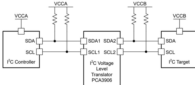
Figure 6-11. PCA9306 I<sup>2</sup>C Voltage Level Translator
