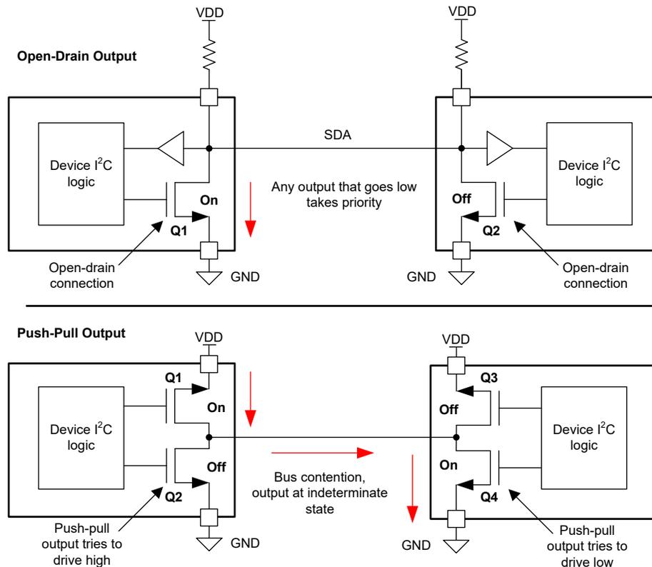
**Figure 2-4. Comparison Between Open-Drain and Push-Pull Contention**
