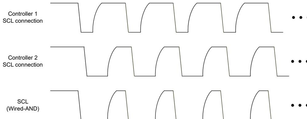
**Figure 6-5. I<sup>2</sup>C Clock Synchronization Resulting Wired-And**
