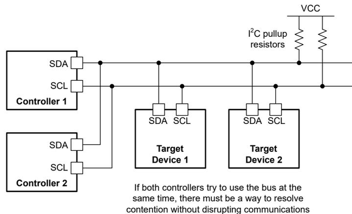
**Figure 6-1. I<sup>2</sup>C Bus Contention With Multiple Controllers**
