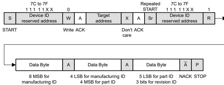
**Figure 5-5. Reading the I<sup>2</sup>C Device ID**
