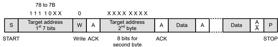
**Figure 5-6. I<sup>2</sup>C Ten-Bit Target Addressing Write**
