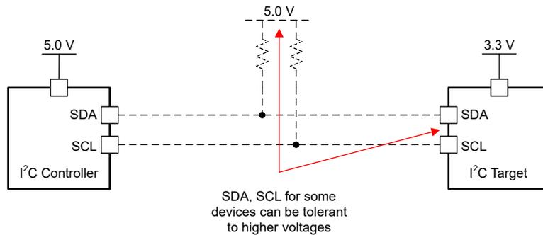
**Figure 6-10. I<sup>2</sup>C Pullup Resistor Over-Driven on Higher-Voltage Tolerant Lines**
