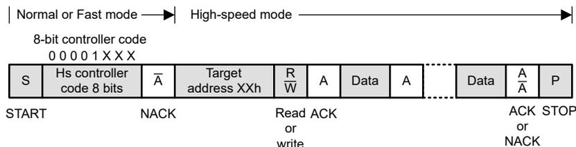
Figure 5-3. Enabling I<sup>2</sup>C High-Speed Mode
