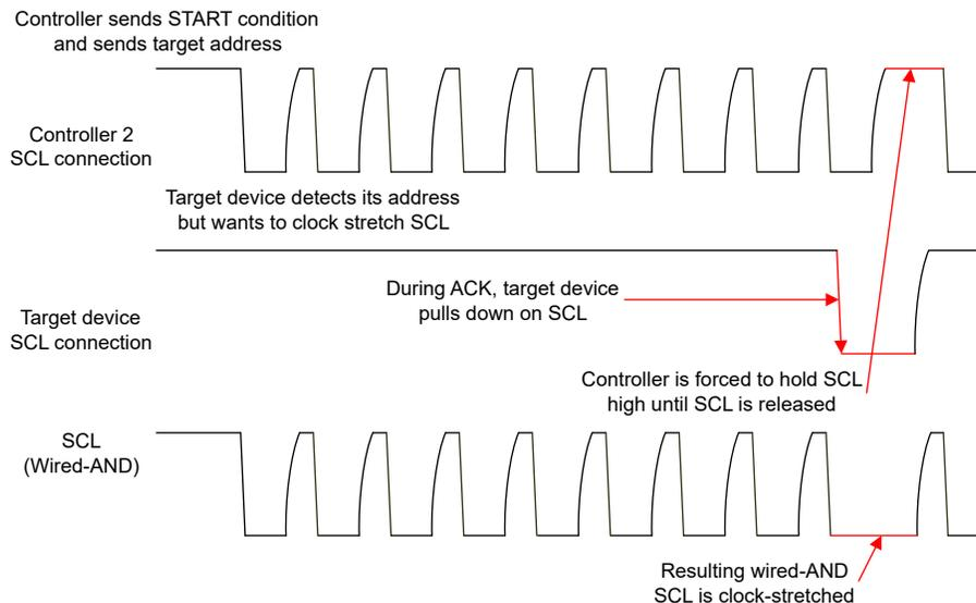
**Figure 6-7. I<sup>2</sup>C Target Clock Stretching**
