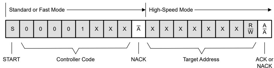
**Figure 5-2. I<sup>2</sup>C High-Speed Controller Code**
