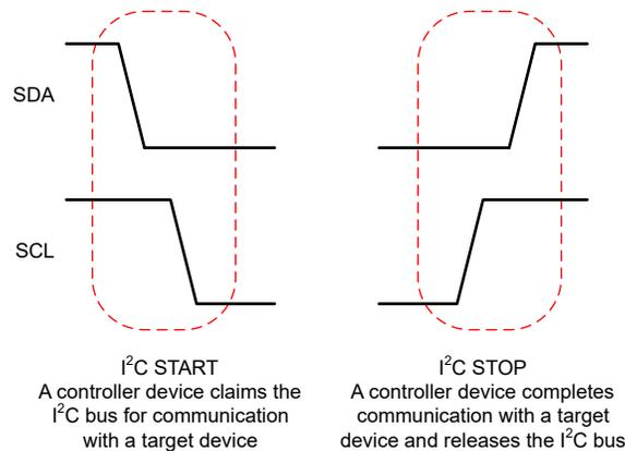
**Figure 3-1. I<sup>2</sup>C START and STOP**
