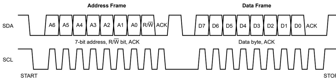
**Figure 3-3. I<sup>2</sup>C Address and Data Frames**
