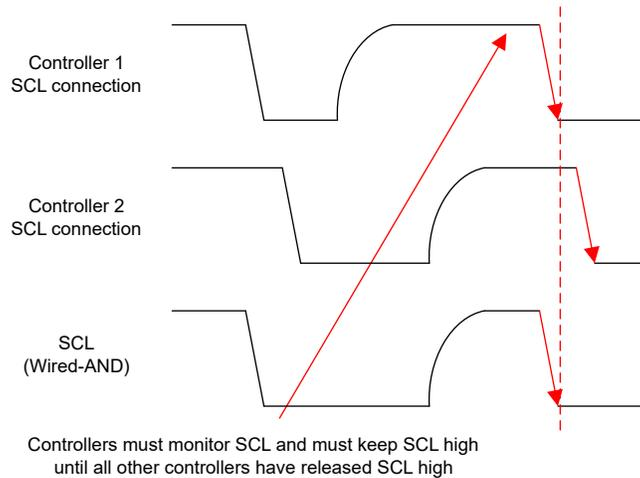
**Figure 6-4. I<sup>2</sup>C Clock Synchronization Monitoring SCL**
