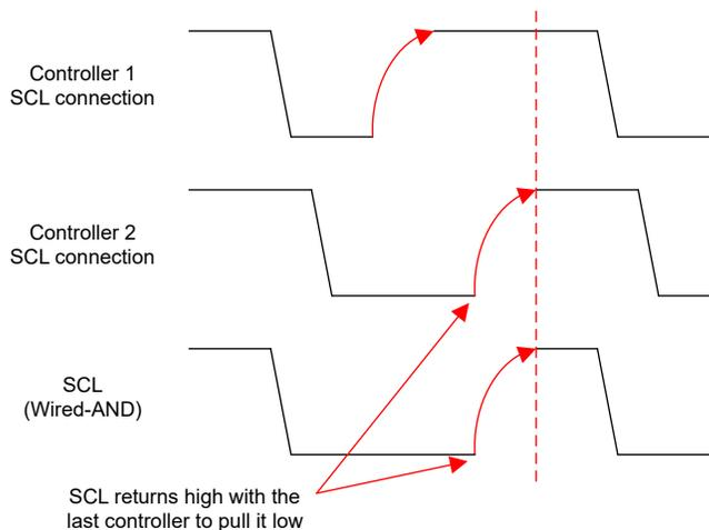
**Figure 6-3. I<sup>2</sup>C Clock Synchronization SCL Returning High**
