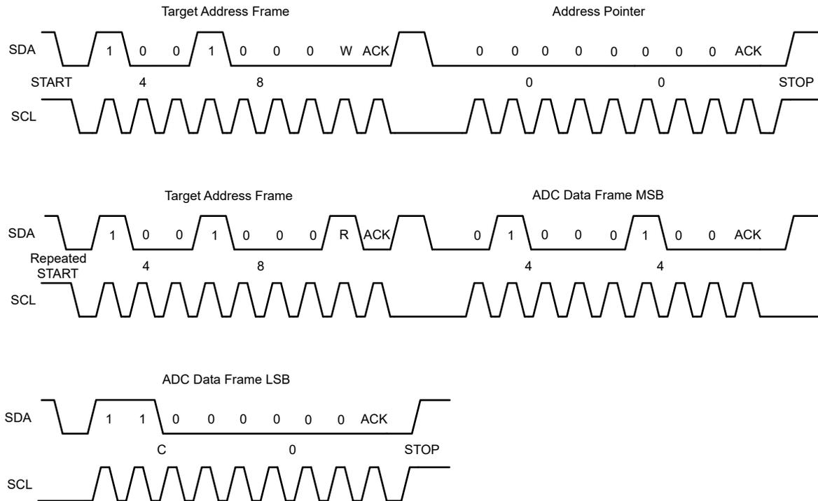
Figure 4-5. I<sup>2</sup>C Transmission for Reading from the ADS1115
