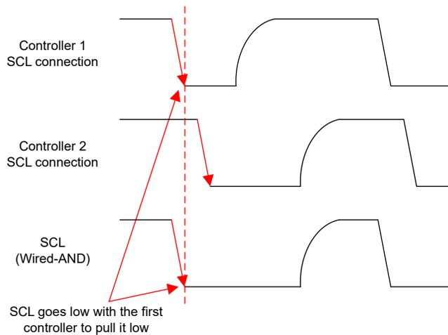
**Figure 6-2. I<sup>2</sup>C Clock Synchronization SCL Going Low**
