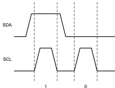
**Figure 3-2. I<sup>2</sup>C Digital One and Zero Representations**
