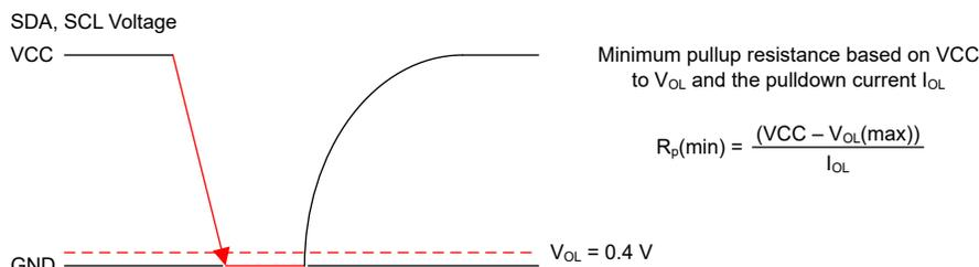
**Figure 6-13. Minimum Pullup Resistance Based on Pull-Down Current**
