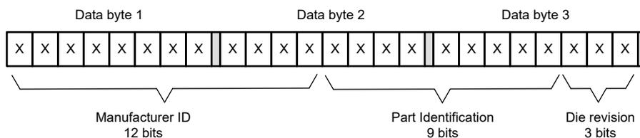
Figure 5-4. I<sup>2</sup>C Device ID Data Bits
