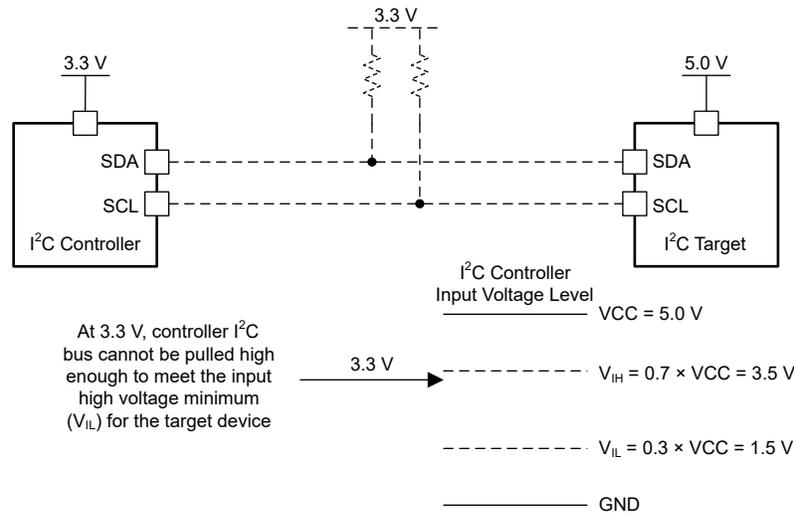
**Figure 6-8. I<sup>2</sup>C Pullup Resistor Under-Drives Inputs on Mismatched Bus Voltages**
