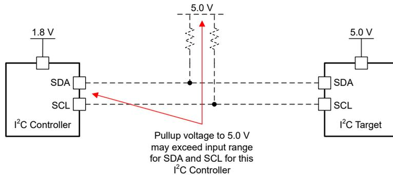
**Figure 6-9. I<sup>2</sup>C Pullup Resistor Over-Drives Inputs on Mismatched Bus Voltages**
